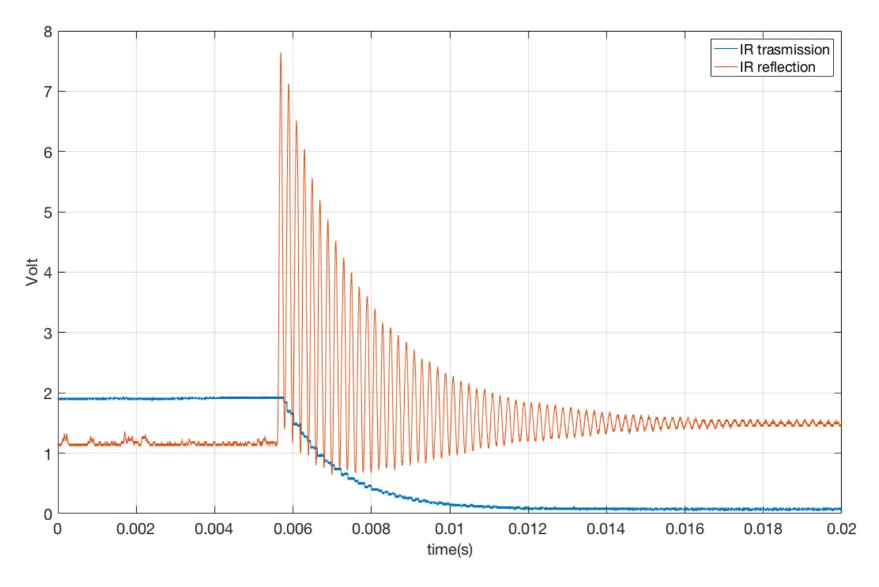
The oscillating transient is possibly due to the servo response to the sudden frequency change.
